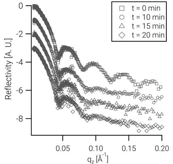
Figure 1: Specular reflectivity of a PS/PMMA bilayer. Fall in intensity of Kiessig fringes attributed to the thinner layer can be observed with increasing annealing time. Curves are offset by factor 10 for clarity reasons.
