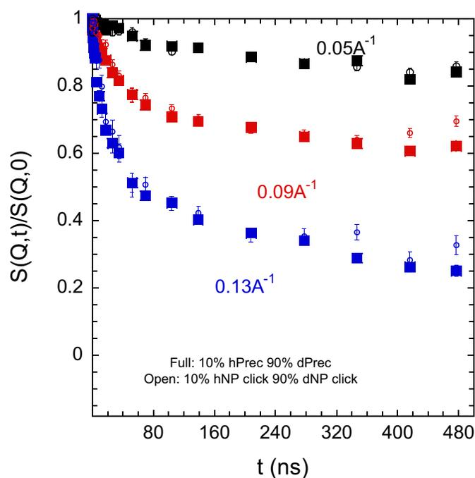
**Figure 2.** Intermediate scattering function obtained by neutron spin echo of 10% hydrogenated linear precursor in deuterated precursor (full squares) and 10% hydrogenated SCNPs in deuterated SCNPs (open circles) at the indicated  $Q$  values.
