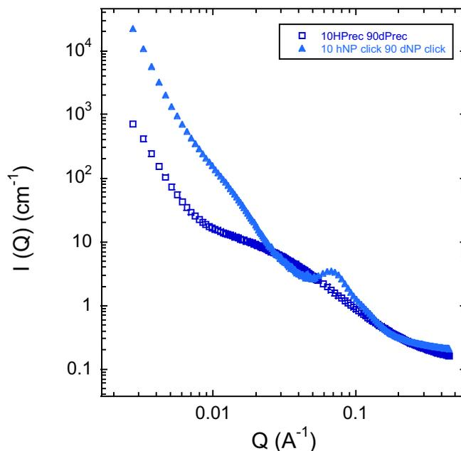
**Figure 1.** Small angle neutron scattering curves of 10% hydrogenated linear precursor in deuterated precursor (squares) and 10% hydrogenated SCNPs in deuterated SCNPs (triangles).
