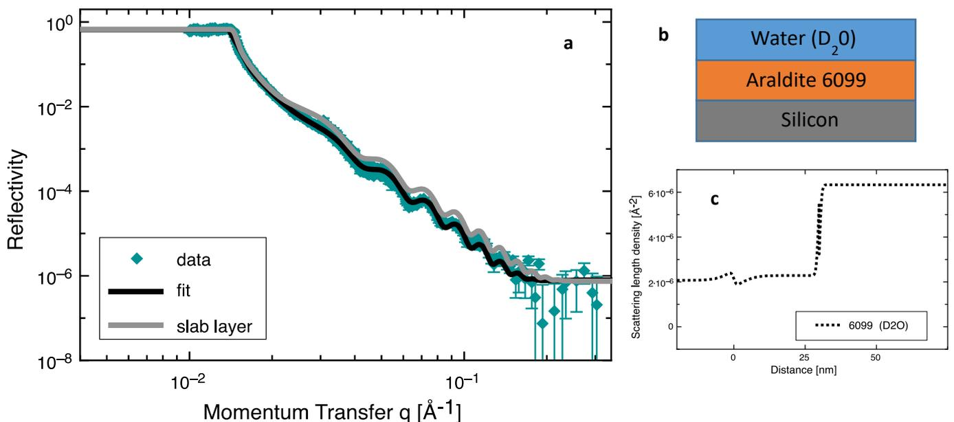
Figure 1: a) Reflectivity data for uncross-linked 6099 epoxy in D<sub>2</sub>O. The included fits are for a slab model which assumes that no D<sub>2</sub>O enters the film and a fit with a graded layer showing the D<sub>2</sub>O profile in the film. b) a diagram which shows the 3 layers used in the fit. c) The SLD profile for the fit showing a depletion layer at the buried interface with a lower concentration of D<sub>2</sub>O.
