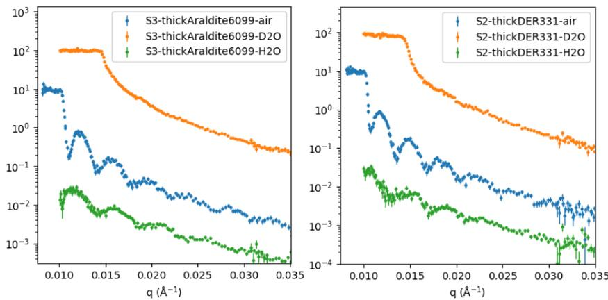
Figure 2: Data for thick films of cross-linked and uncross-linked epoxy in air, D<sub>2</sub>O and H<sub>2</sub>O. In D<sub>2</sub>O the films ended up contrast matched to the Silicon resulting in the loss of fringes
