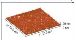
**Figure 1:** AFM image of partially oxidised cellulose film, roughness 1.3nm
