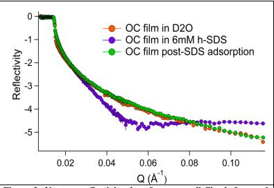
Figure 2: Neutron reflectivity data for an oxcell film before and after SDS adsorption followed by washing with  $D_2O$
