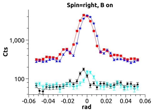
**Figure 6:** Rocking curve of the same magnetite NPC grating as in Fig. 3 with the electromagnet turned on for spin "right". Note that the small asymmetry in the peak heights of the  $\pm 2$  diffraction orders is inverted as compared to Fig. 5.
