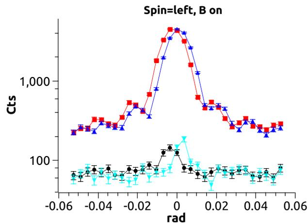
**Figure 5:** Rocking curve of the same magnetite NPC grating as in Fig. 3 with the electromagnet turned on for spin "left". Note the small asymmetry in the peak heights of the  $\pm 2$  diffraction orders.
