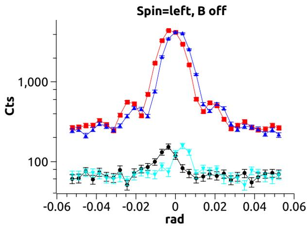
**Figure 3:** Rocking curve of a magnetite NPC grating (thickness  $\approx 33 \mu\text{m}$ , grating spacing =  $0.5 \mu\text{m}$ ) with the electromagnet turned off for spin "left".
