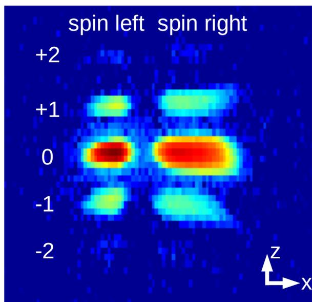
**Figure 2:** A typical detector image as obtained only using SG (P was not used) and the sample in place at a particular  $\theta$ . The diffraction spots corresponding to one spin direction are arranged vertically in two columns. The various diffraction orders of the grating ( $-2, \dots, +2$ ) are observed in five rows.
