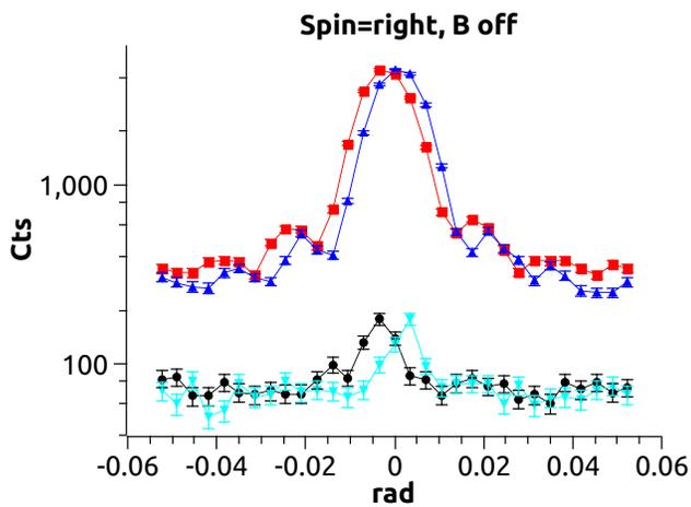
**Figure 4:** Rocking curve of the same magnetite NPC grating as in Fig. 3 (with the electromagnet turned off also) for spin "right". The curves are practically identical to what is shown in Fig. 3.
