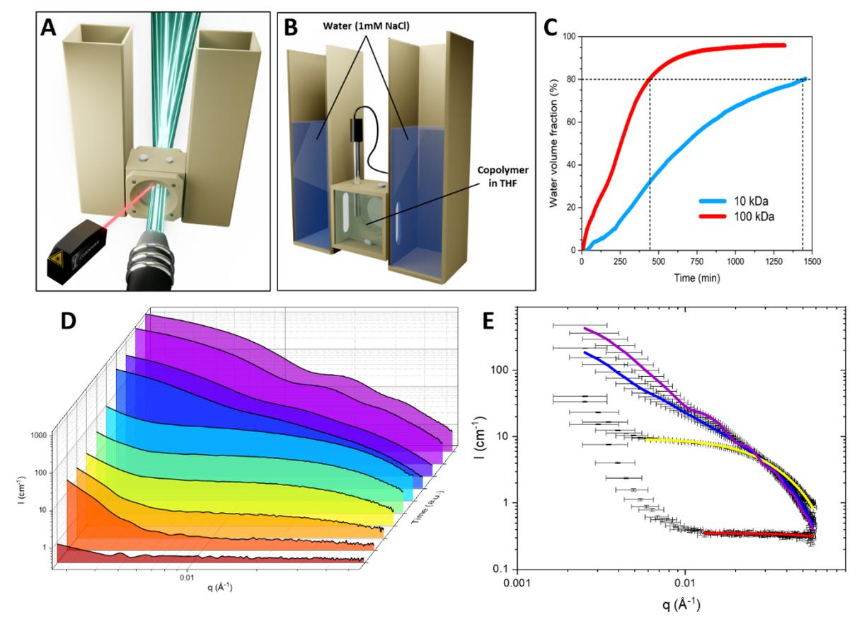
**Figure 1.** A- Dialysis cell used on D22 to monitor the step-by step formation of Block Copolymer (BC) vesicles. A remote-head DLS set-up could be used as well. B- The 4 ml cell containing the non-interacting BCs in d8-THF is sandwiched between two D<sub>2</sub>O reservoirs containing 1 mM NaCl in order to continuously monitor the cell conductivity and then the exact water
