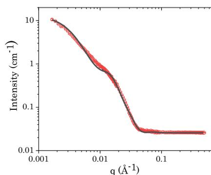
Figure 2: SANS scattering curves of post Mb-Psomes in the collapsed state at 0.1  $\text{mg mL}^{-1}$ . Solid line represents fitting curve based on the vesicle model.
