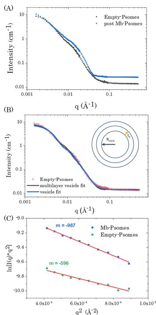
**Figure 3: (A) SANS scattering curves of empty-Psomes and Mb-Psomes (BCP-AS109) in the collapsed state; (B) Model fits of the empty-Psomes using two different models. (C) Kratky-Porod plot for empty and loaded polymersomes in D<sub>2</sub>O. Conditions:  $c_{BCP} = 0.1 \text{ mg mL}^{-1}$ .**
