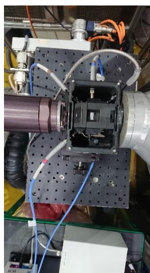
Figure 2. NUrF setup from above without the top cover. The cuvette is visible in the centre and around the fibre optics and the neutron beam nozzle.
