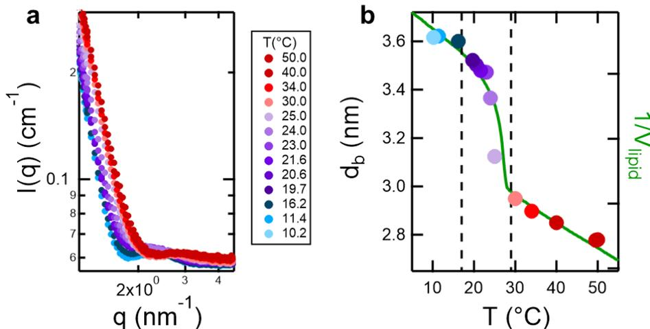
**Fig. 1** Temperature dependence of (a) the high  $q$  SANS data and (b) corresponding bilayer thicknesses ( $d_b$ ) determined by fitting the data with a vesicle form factor. The green line in (b) shows that the changes in  $d_b$  directly follow the changes in lipid volume measured with densitometry. The red, purple, and blue symbols correspond to temperatures in the fluid phase, melting transition, and gel phase, respectively.
