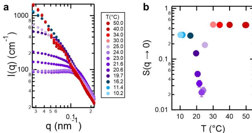
**Fig. 2** Temperature dependence of (a) low  $q$  SANS data and (b) extrapolated  $S(q \rightarrow 0)$ . Values for  $S(q \rightarrow 0)$  were determined by dividing the measured SANS data by the calculated vesicle form factor. The red, purple and blue symbols correspond to temperatures in the fluid phase, melting transition and gel phase, respectively.
