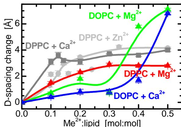
**Figure 3:** Changes to the transversal lamellar D-spacing in the various multilayered model membranes studied. The changes appear to group by lipids (i.e., DOPC vs. DPPC) rather than by the cations added (i.e., Ca<sup>2+</sup>, Zn<sup>2+</sup>, and Mg<sup>2+</sup>).
