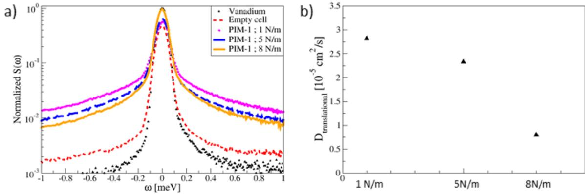
Figure 2: a) Quasi-elastic spectra of the vanadium, the empty cell and of the PIM-1 sample at three different mechanical stresses under constant hydraulic pressure (14 bars) b) Translational motion of the confined water
