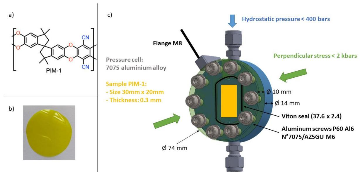
Figure 1: a) PIM-1 structure b) PIM-1 sample c) Homemade aluminium pressure cell. The mechanical stress ( $< 2$  kbars) is applied ex-situ with a torque wrench ensuring a proper tightening level (to a fixed torque value) of the screws.
