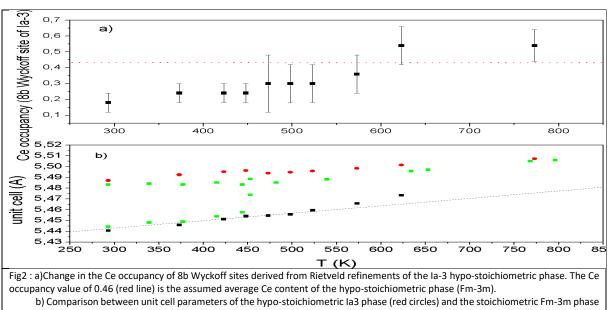
(black squares) at all temperatures studied (the dotted is a fit through unit cell parameter values of the  $U_{0.56}$ Ce<sub>0.44</sub>O<sub>2</sub> Fm-3m phase). The unit cell parameter values for the two phases (for a similar overall oxygen content) reported in the literature [1,2] are also plotted (green squares).
