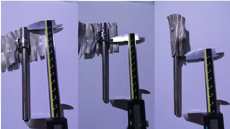
Fig. 1. ThO 2 sample in the ZrY 4 container with its Al sample holder wrapped in a Cd foil.
