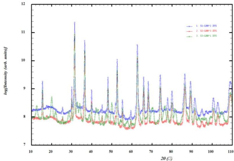
Furthermore, *ex situ* samples of cycled electrodes were measured. Although signal-to-noise ratio is much lower for these *ex situ* samples they contain valuable information on the reversibility of electrochemical mechanism and material degradation. By comparing their diffraction pattern with those of pristine materials we observe that spinel phase as well as TM ordering are maintained throughout repeated electrochemical lithiation and delithiation.
