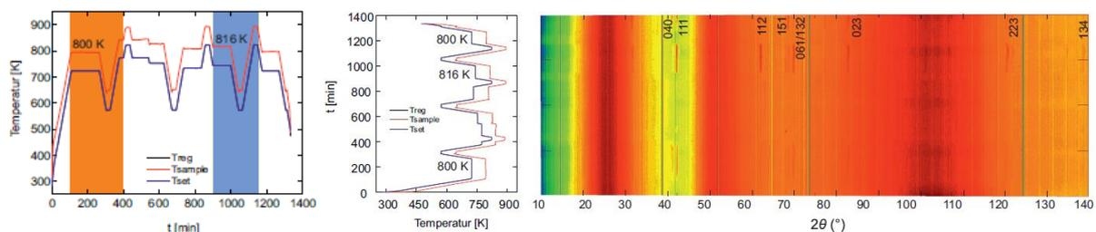
**Fig. 2.** Full temperature program applied to the ampoule of Figure 1. The blue line is the set temperature of the oven, the red line is the sample temperature, derived by temperature calibration of an ex situ  $\text{NaCl/KCl}$  measurement. The orange and blue area are taken into account for further discussions. Black phosphorus is formed upon heating to 800 K (orange) and is condensed from the gas phase (blue). Color coding of the intensity: blue (low) to red (high).
