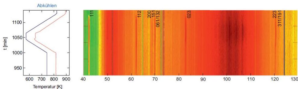
**Fig. 4.** Section of the temperature program applied to the ampoule of Figure 1 (blue part of Fig. 2) and neutron powder diffractograms for the isothermal black phosphorus formation at 816 K. Formation of black phosphorus by cooling a phosphorus gas phase down to 816 K. Color coding of the intensity: blue (low) to red (high).
