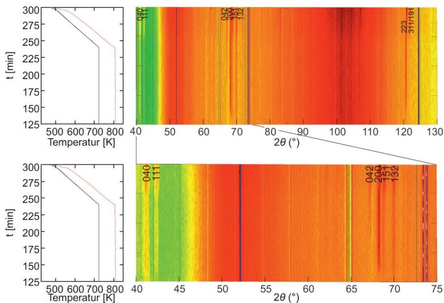
**Fig. 5.** Section of the temperature program applied to a 7.1 cm ampoule loaded with 400 mg of red phosphorus, 16 mg Sn and 8,032 mg SnI<sub>4</sub>. Neutron powder diffractograms for the isothermal black phosphorus formation at 807 K. Formation of black phosphorus by heating the mixture to 807 K. Color coding of the intensity: blue (low) to red (high).
