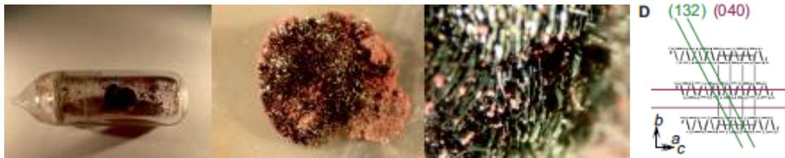
**Fig.1.** 4 cm silica glass ampoule containing red phosphorus, tin and  $\text{SnI}_4$  starting materials. The mixture was fully reacted to the final product black phosphorus, measured at various temperatures. Middle: Bulk residue and layered crystals of black phosphorus covered by orange spots of  $\text{SnI}_4$ . Crystal structure section of black phosphorus with a view parallel the phosphorene sheets. (040) and (132) layers are given.
