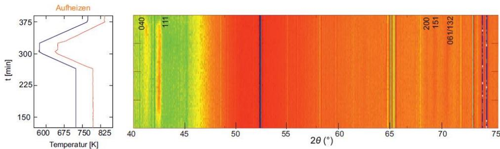
**Fig. 3.** Section of the temperature program applied to the ampoule of Figure 1 (orange part of Fig. 2) and neutron diffractograms for the isothermal black phosphorus formation at 800 K. Indices of the reflections are given. Non-indexed events and spots are due to detector faults and the silica glass ampoule. Color coding of the intensity: blue (low) to red (high).
