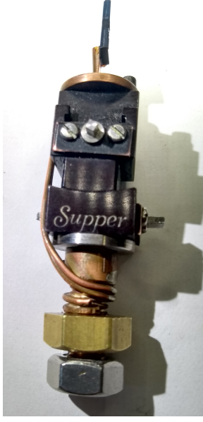
(a) Sample attached to copper post on mini-goniometer connected with two 1 mm 2 copper wires to the cryostat sample rod.
