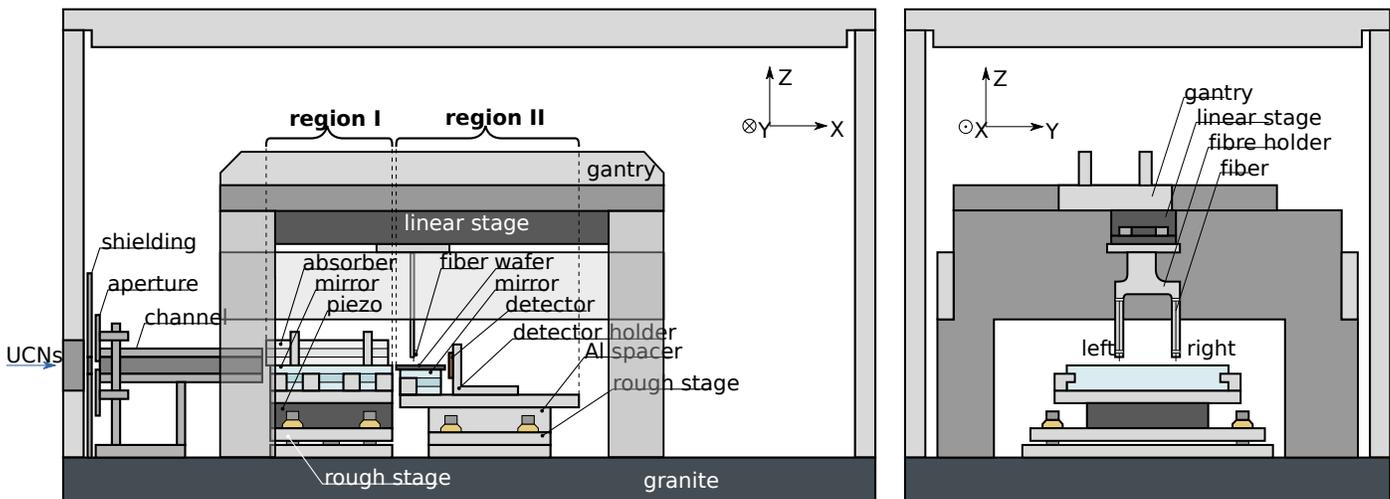
Figure 1: Experimental setup used for all measurements during DIR-245. Left: side view; Right: cut view at the position of the detector. Graphics courtesy of Janik Trauner.
