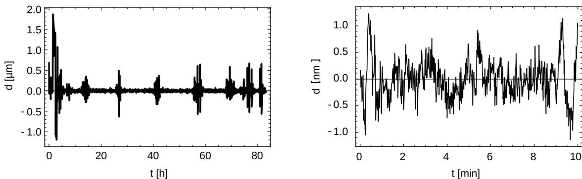
Figure 3: Interferometric measurements. Left: Continuous measurements with active PID feedback. At around 9:00 in the morning and in the evening each day during the week, strong vibrations occurred on Niveau D, which are visible as disturbances. Right: Interferometer stability in a temperature-controlled vibration isolated environment (post beamtime). Graphs courtesy of Janik Trauner
