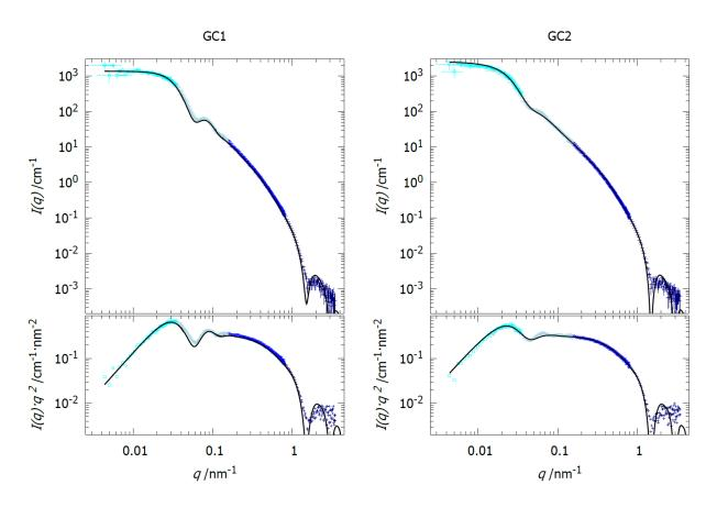
Analysis: A model of two population of uni- and bilamellar spherical vesicles, with a common hard sphere structure factor of corresponding number density, was used. The shell thickness was found to be 42 nm for one lamella, with 15 % (by number) liposomes having 2 lamella. The mean core radii are 47 and 56 nm for GC1 and 2 respectively, with relative standard-deviations of 0.20 and 0.33 respectively.
