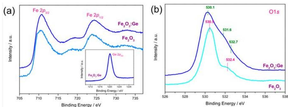
Figure 2 – X-ray absorption spectra of the Fe 2p (a) and O 1s (b) core levels for both  $\text{Fe}_2\text{O}_3$  and  $\text{Ge}:\text{Fe}_2\text{O}_3$  compositions; in the insert the Ge 2p core level for the doped system.
