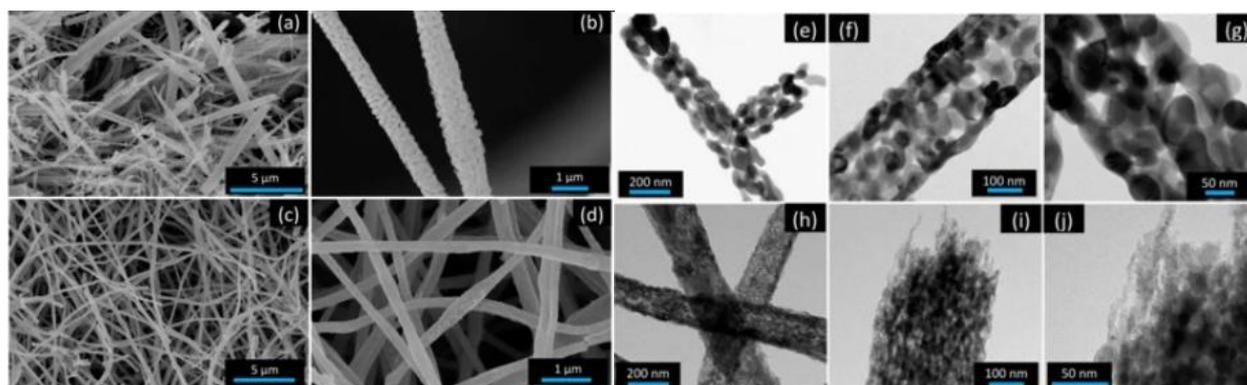
Figure 1 SEM images (a-d) and TEM images (e-g); SEM images (a,b) of the  $\text{Fe}_2\text{O}_3$  reference compound and (c,d) for the Ge: $\text{Fe}_2\text{O}_3$  system; TEM images (e-g) of the  $\text{Fe}_2\text{O}_3$  reference compound and (h-j) for the Ge: $\text{Fe}_2\text{O}_3$  system.
