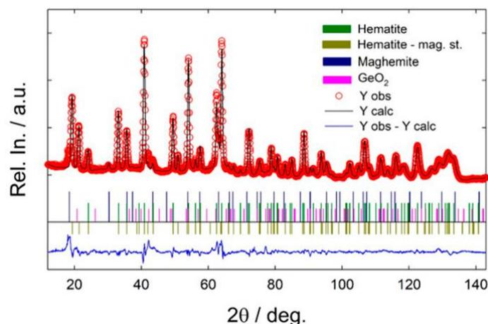
Figure 3 – Rietveld refinement of the powder diffraction pattern of  $\text{Ge}:\text{Fe}_2\text{O}_3$  system ( $\chi^2 = 22.0$ ,  $R_p$ , 1.97,  $R_{wp} = 2.39$ ); phase composition has been identified: hematite 91.1%, maghemite 8.6 %,  $\text{GeO}_2$  0.3%
