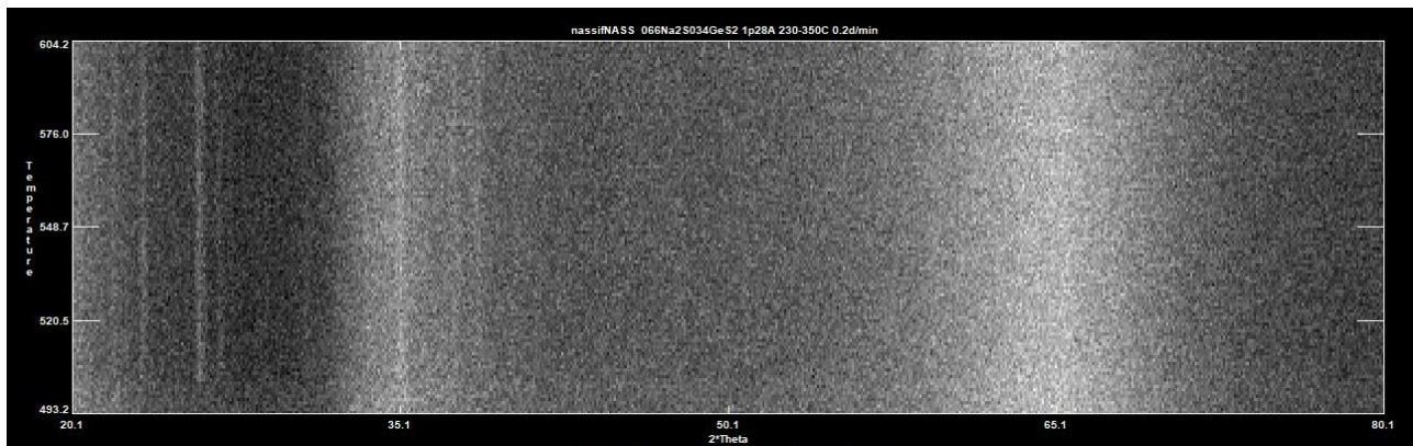
Figure 1: 2D plots of the powder thermodiffractograms for the 0.66\text{Na}_2\text{S}-0.34\text{GeS}_2 sample.
