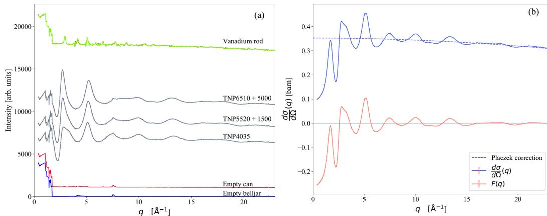
Figure 1: (a) Raw data from the vanadium rod, the empty instrument, the empty can and the three TNP samples. The data for the TNP5520 and TNP6510 has been shifted up for visualization purposes but both oscillate around the same intensity level as the TNP4035 sample. (b) TNP4035 sample corrected for (top) background, attenuation and multiple scattering and (bottom) Placzek. All data is plotted with its corresponding errorbars that are however too small to be visible at this scale.
