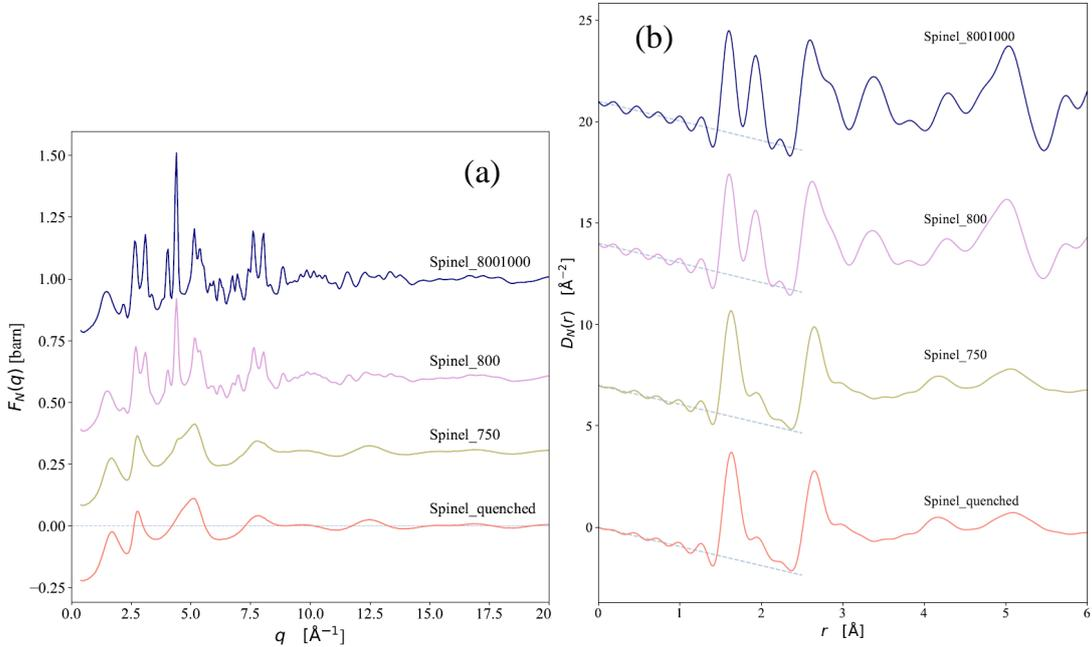
Figure 3: (a)  $F_N(q)$  for the Spinel glass ceramics. All the functions oscillate around zero but Spinel\_750, Spinel\_800 and Spinel\_8001000 have been shifted up for clarity. (b)  $D_N(r)$  for the Spinel glass ceramics. Notice how all the functions oscillate around the density line  $-4\pi nr$  at low  $r$ . This is used as a consistency to check to verify the accuracy of the corrections performed.
