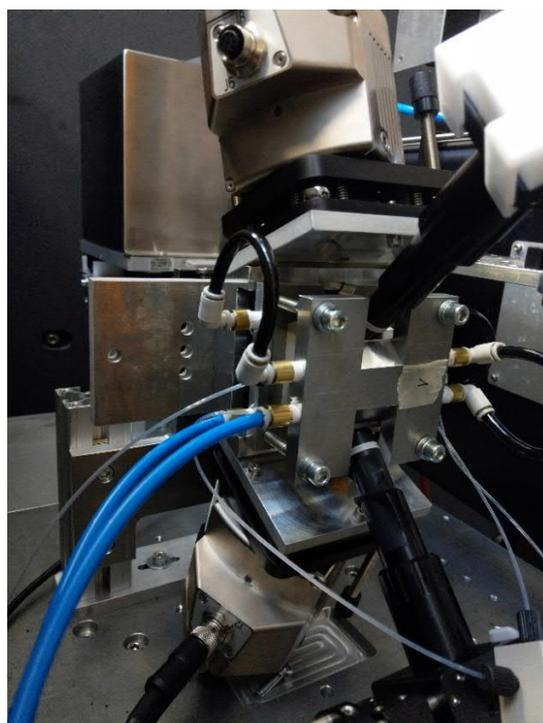
**Fig. 6:** Installation of the mobile ATR-IR/SE setup on FIGARO (left) and D17 (right). The lower two photos each show a magnified view of the liquid flow cell with IR beam path, and SE light source and detector, respectively.
