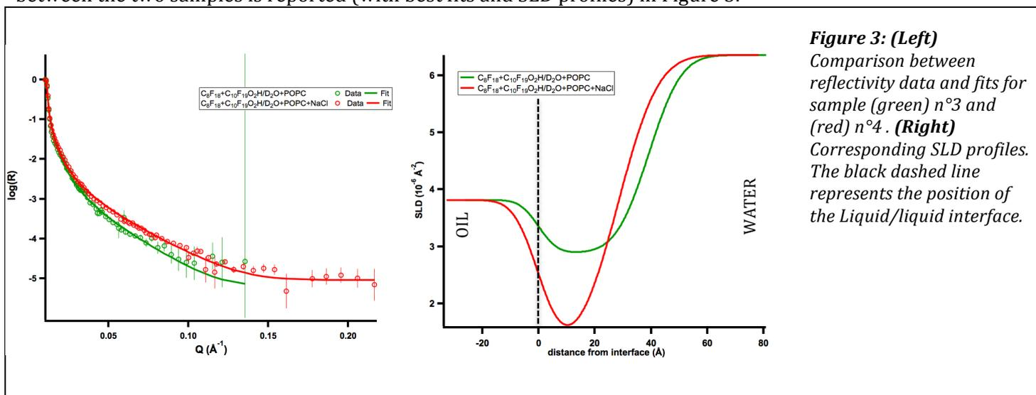
**Figure 3: (Left)** Comparison between reflectivity data and fits for sample (green) n°3 and (red) n°4. **(Right)** Corresponding SLD profiles. The black dashed line represents the position of the Liquid/liquid interface.
