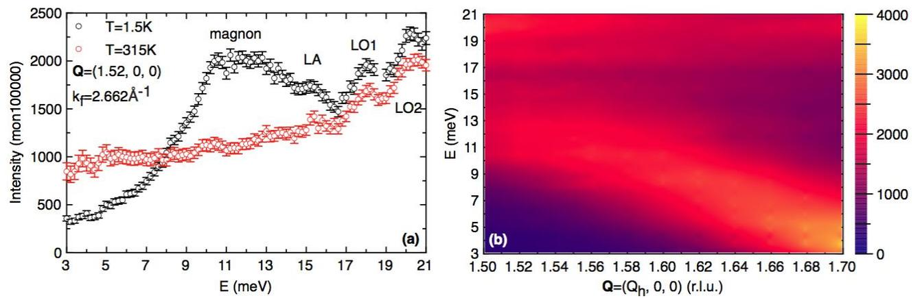
**Fig. 1:** (a) Energy spectra at  $Q=(1.52, 0, 0)$  measured at IN8 spectrometer with unpolarized setup at 313K (red circles) and 1.5K (black circles). The measured intensity for the spectrum collected at  $T=315\text{K}$  is corrected by the Bose factor. (b) Colour map constructed from E scans around  $(2\ 0\ 0)$ . Data were collected at  $T=1.5\text{K}$ .
